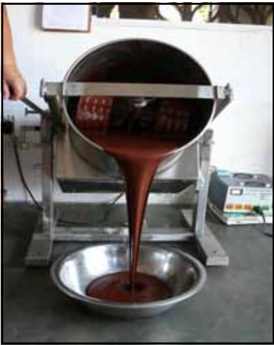
Conch machine: velvety smooth and rich but still not finished
